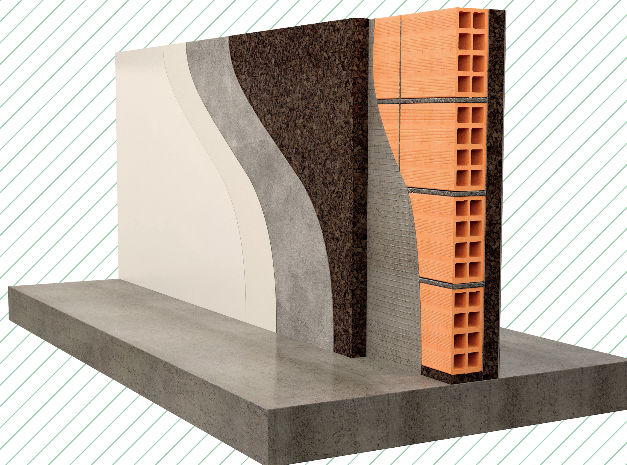
④ INTERNAL PARTITIONS WITH INSULATION LINED ON BOTH SIDES
