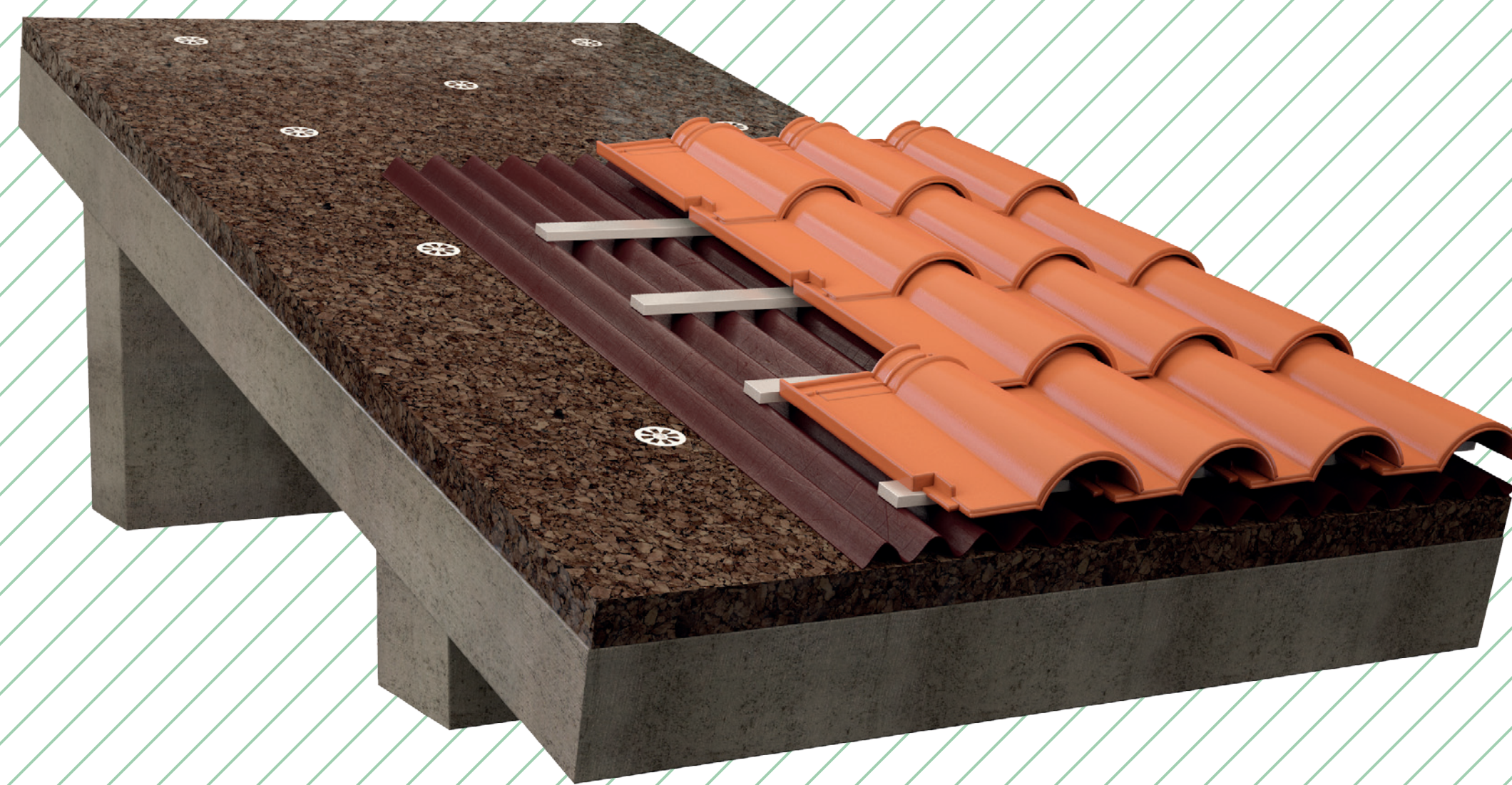
④ PITCHED ROOF WITH CORRUGATED ROOFING SYSTEM
